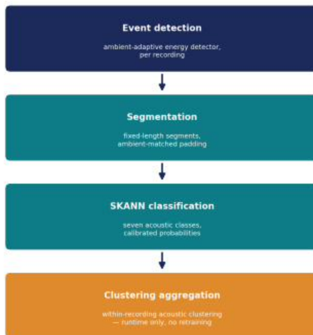
Left: class territory map — UMAP projection of the learned embedding space, with Voronoi territories drawn from class centroids (backbone stage, four acoustic superclasses). Sources separate cleanly in the space the network learns. Right: the PS12 inference pipeline.
